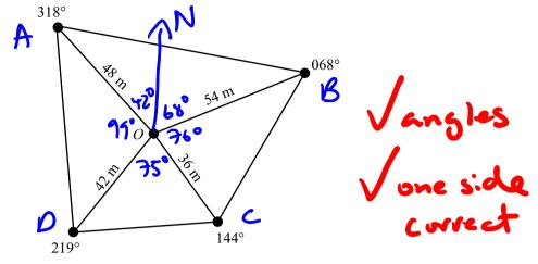
The information from a compass radial survey of a field is shown in the diagram above.
