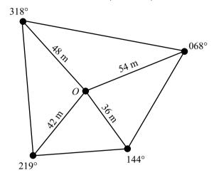
The information from a compass radial survey of a field is shown in the diagram above.
