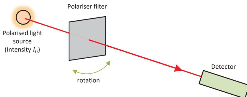
The student begins with a polarised light source of intensity  $I_0$ . They adjust the polarising filter until the maximum amount of light passes through it, and set this angle equal to zero. Then, they adjust the angle of the filter relative to this, and record the amount of light that passes through. Their data is recorded in the table below.
