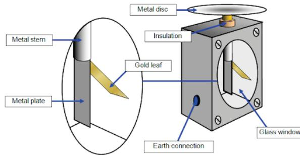
A zinc plate is attached to the top of the electroscope and the electroscope is given a net negative charge; this puts the gold leaf in an outward position. Two different coloured lights are shone on it separately.
