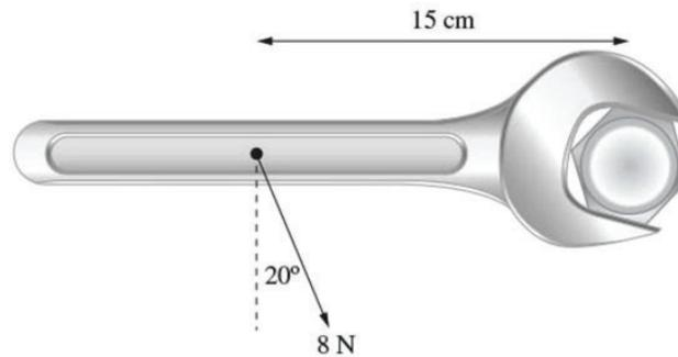
The torque being applied to the bolt by the spanner is:
