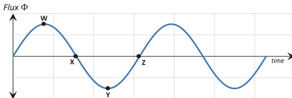
At which point(s) in the rotation is the magnitude of the induced voltage greatest?
