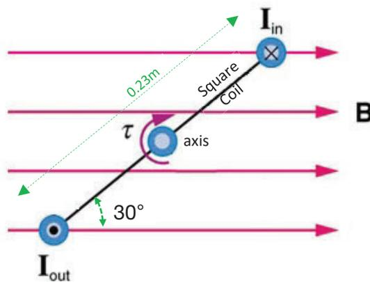
The square coil consists of 8 turns of wire, and has dimensions  $0.23 \times 0.23$  m. A current of  $I = 2.75$  A flows through it. The external magnetic field is  $B = 1.50$  T
