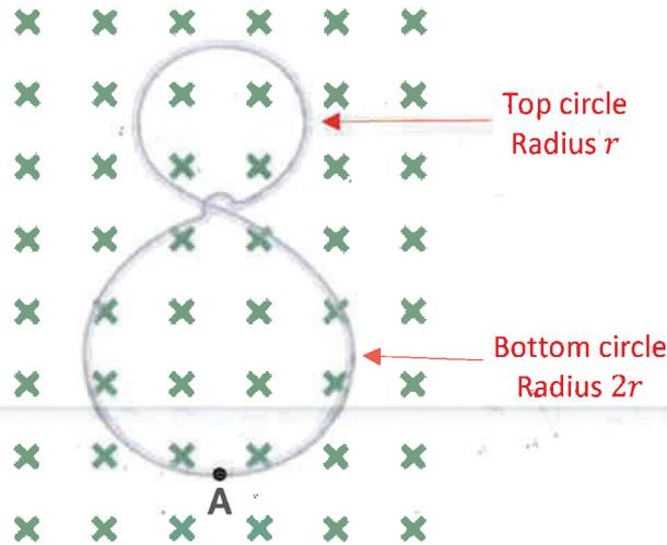
A uniform magnetic field is applied perpendicular to the plane of the two circles, in the direction shown. The magnetic field is increasing at a constant rate.
