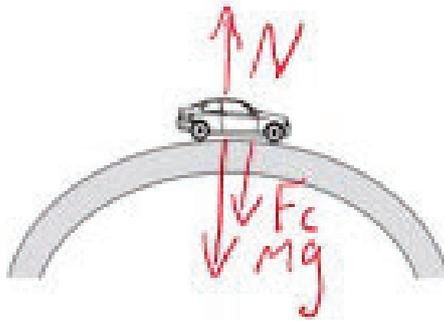
He noticed that the reading on the scales decreased as he passed over the top of the bridge. He claimed later to a friend that if he could have travelled fast enough, the scales would have registered zero.
