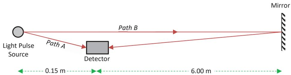
The detector is a photocell that converts the light into a photocurrent. The photocell can only record received signals, so there is no way to know on the graph when the pulse was sent. After the detector was set to record, the times at which the light from each path are received are shown in the graph below.
