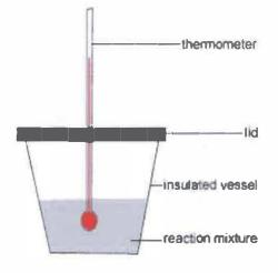
10.0 mL of 0.500 M solution of HCl are mixed with 10.0 mL of 0.500 M solution of NaOH in the cup shown. The enthalpy change for this reaction is -55.8 kJ mol<sup>-1</sup>.
