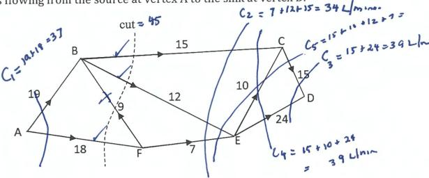
(a) What is the capacity of the cut shown in the diagram?
