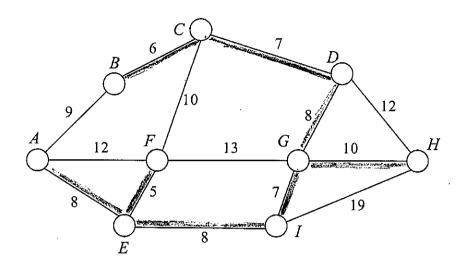
(a) A minimum spanning tree is going to be used by the engineers to lay the cables to connect all towns by underground fibreoptic cable running on the side of the roads. Calculate the minimum length of the fibreoptic cable that needs to be laid to connect all the towns. Show all necessary working.
