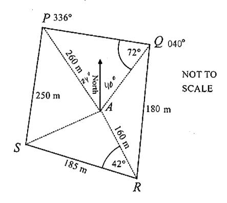
The bearing from A of P is  $336^{\circ}$  and of Q is  $040^{\circ}$ , and the distance AP is 260 m.
