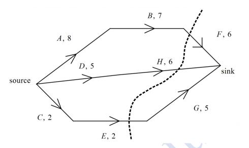
a) Determine the capacity of the cut.
