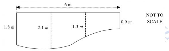
Use three applications of the trapezoidal rule to determine the approximate capacity of the pool, in litres.
