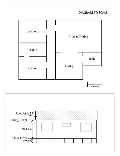
(a) Use the scale given on the floor plan to calculate the total length (perimeter)2 of the outer walls of the house. Give your answer in metres.
