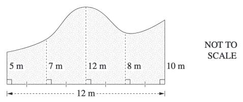
Find the area of the field, using two applications of the trapezoidal rule.
