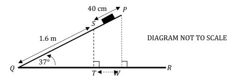
When the coin reaches the point S on the ramp 40 cm from P, it has 1.6 m to slide to reach Q.
