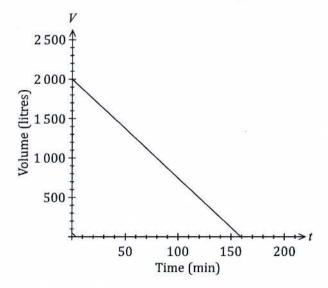
What is the constant rate at which the water is being pumped out of the tank?
