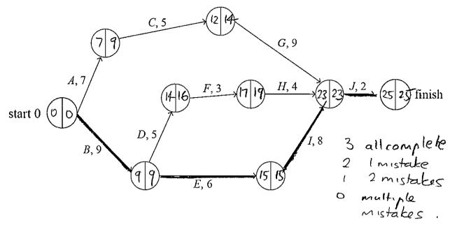
(i) Write the earliest starting times (ESTs) and latest starting times (LSTs) on the above network diagram.
