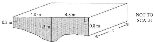
(i) Use two applications of the trapezoidal rule to show that the area of the cross section is approximately 9 m<sup>2</sup>.
